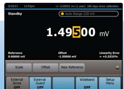
OFFSET and SCALE keys make it easy to compensate for zero offset and scale errors and permit direct display of linearity errors at any scale level.
