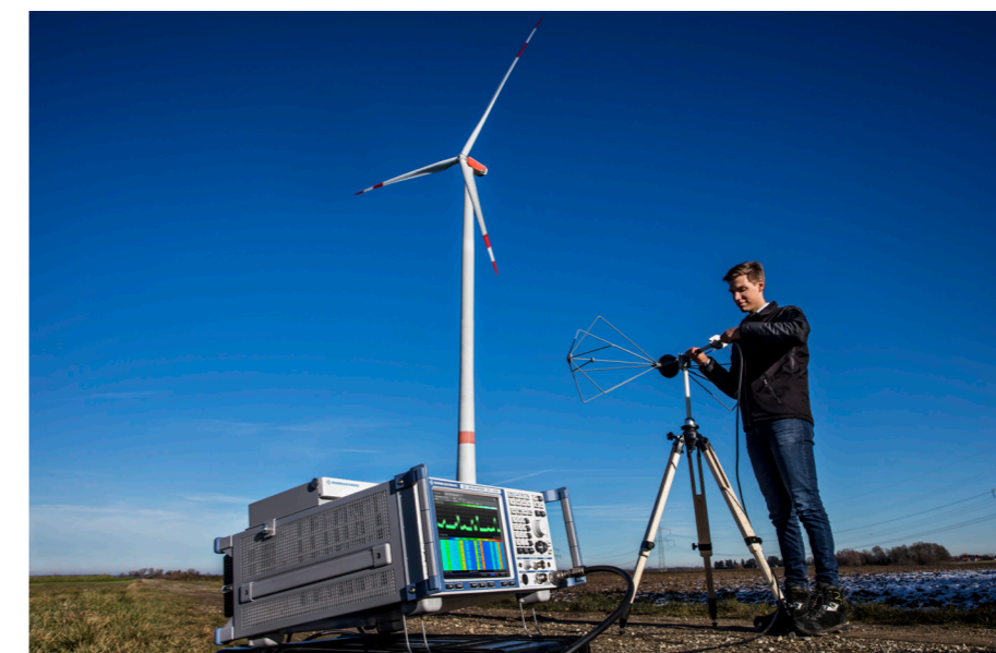
Battery-operated in-situ measurements with the R&S®ESR.
