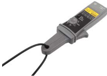
Figure 2 Connection between the Test Clamp and Conductor
