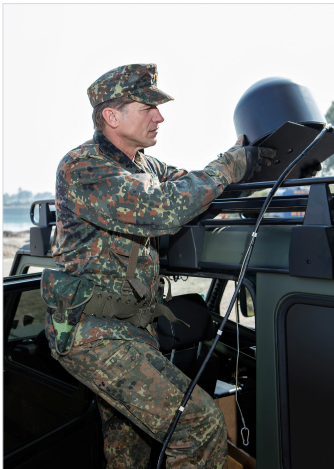
Automatic direction finding with Rohde&Schwarz compact DF antennas on a magnet mount (requires R&S®PR300-DF option).
